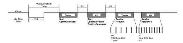
The timing values for the fast initialisation and communications in general are detailed in the tables below. There are different possibilities for the idle time:
