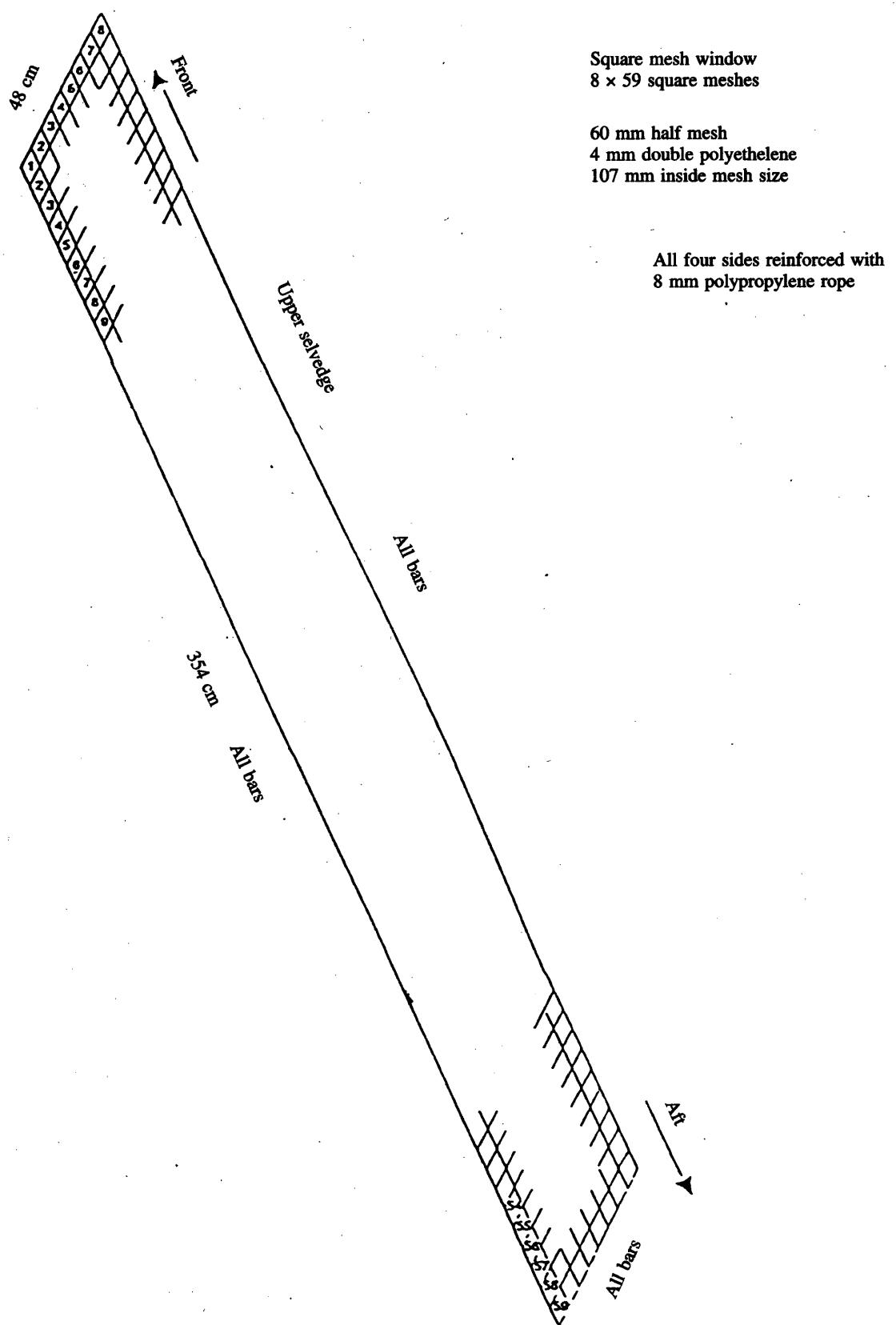
*Figure 3***Inserting the window in the cod end****A suggested specification**
