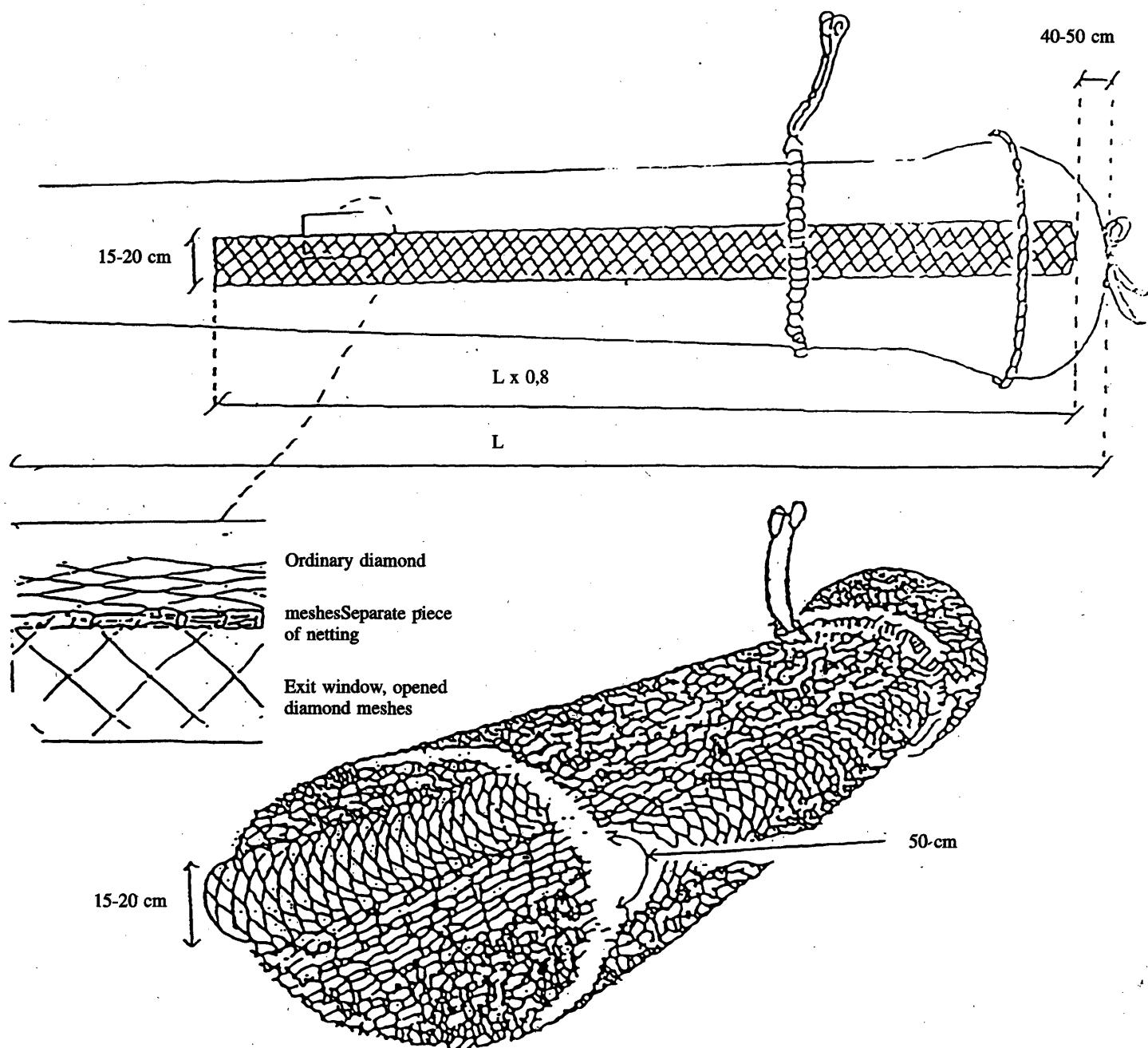
*Figure 1***Position of the square mesh windows in the cod end**
