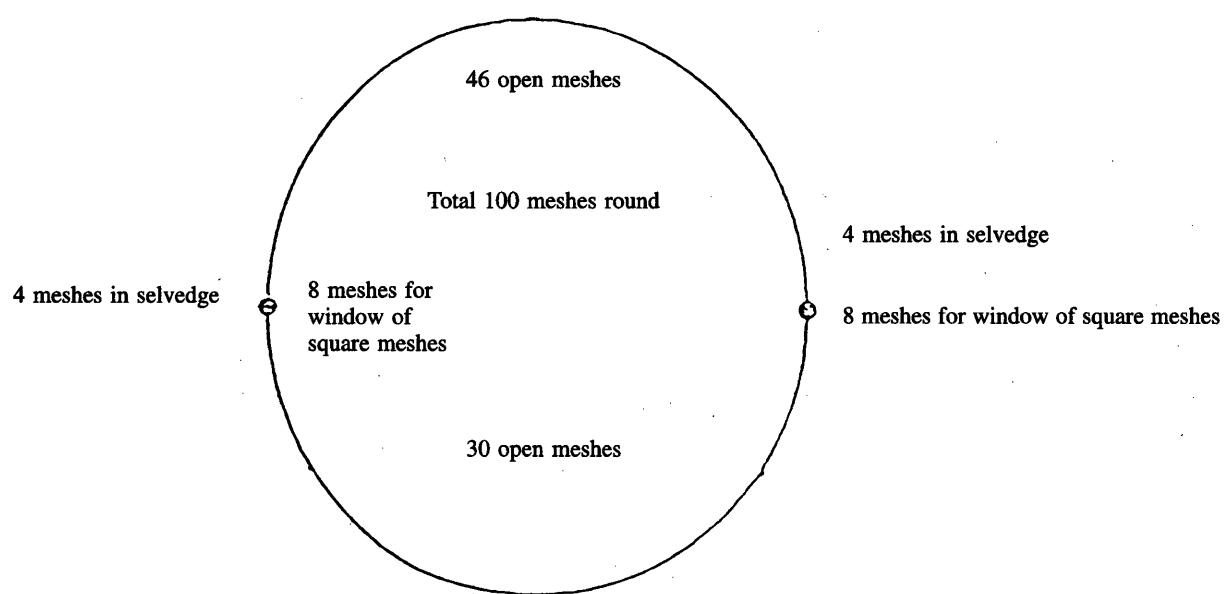
*Figure 2***Netting in the square mesh windows****A suggested specification**
