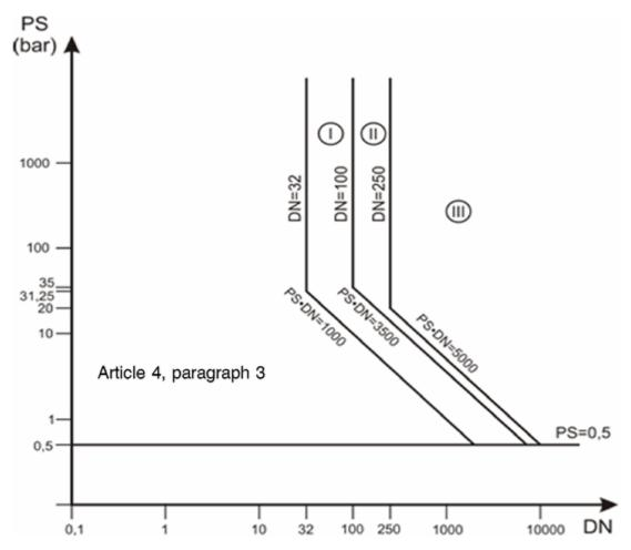
Exceptionally, all piping containing fluids at a temperature greater than 350 °C and falling within category II on the basis of Table 7 shall be classified in category III.
