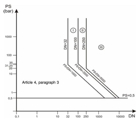
Exceptionally, all piping containing fluids at a temperature greater than  $350\,^{\circ}\text{C}$  and falling within category II on the basis of Table 7 shall be classified in category III.
