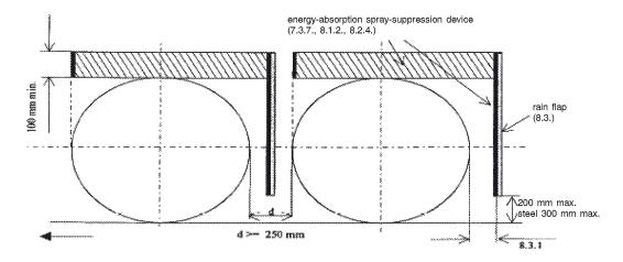
(b) Single axles or multiple axles where the distance between the tyres is not less than 250 mm.
