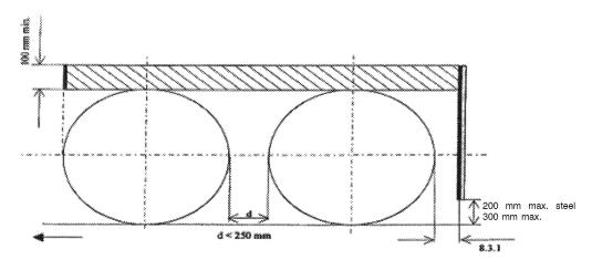
(a) Multiple axles where the distance between the tyres is less than 250 mm.
