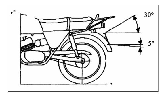
$\label{eq:Figure 1} Figure \ 1$  Angle of geometric visibility (dihedral with horizontal edge)
