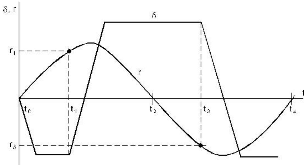
$t_0$  = Start of evasive action manoeuvre $t_1$  = Time to reach turning speed  $r_1$  $t_2$  = Time to reach turning speed  $r_2 = 0$  $t_3$  = Time to reach turning speed  $r_3$  $t_4$  = Time to reach turning speed  $r_4 = 0$  (end of evasive action manoeuvre) $\delta$  = Rudder angle [°] $r$  = Turning speed [°/min]
