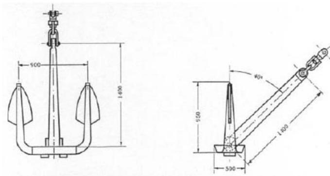
A tolerance of  $\pm 5\%$  applies to the dimensions and mass given. However, the surface area of each fluke must be at least  $0,15\text{ m}^2$ .
