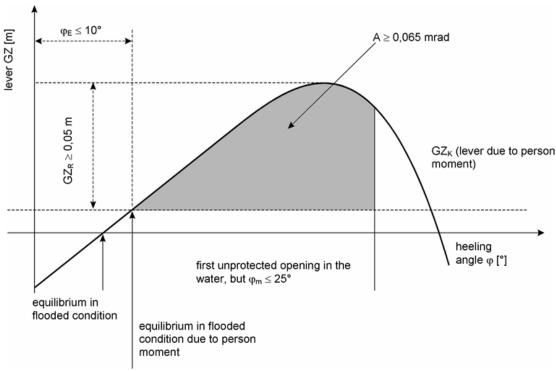
$$\overline{KG}_{Zul} = \frac{\overline{KM} - \frac{I - i}{2\forall} \left(1 - 1.5\frac{F}{F}\right) + 0.75\frac{B_{WL}}{F} \left(Z \cdot \frac{T_m}{2} - h_{KW} - h_{KfO}\right)}{0.75 \cdot \frac{B_{WL}}{F} \cdot Z + 1} \left[m\right]$$
