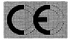
If the CE marking is reduced or enlarged the proportions shown in the above drawing must be respected.
