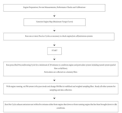
One or more practice cycles may be run as necessary to check engine, test cell and emissions systems before the measurement cycle.
