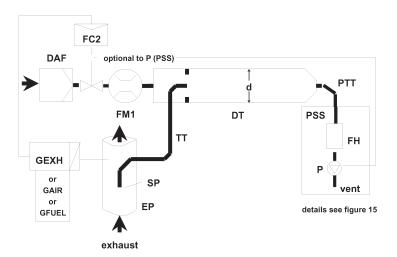
Raw exhaust gas is transferred from the exhaust pipe EP to the dilution tunnel DT through the sampling probe SP and the transfer tube TT. The total flow through the tunnel is adjusted with the flow controller FC3 and the sampling pump P of the particulate sampling system (Figure 16).
