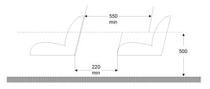
$\label{eq:Figure 4} Figure \ 4$  Determination of unobstructed access to door
