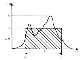
2.6. Clamping force F<sub>c</sub> is the arithmetical mean value of the effective forces, measured at the same measuring point subsequently more times:
