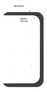
$Figure\ 18$  Permitted intrusion of a wheel arch not extending beyond the vertical centre line of the side seat
