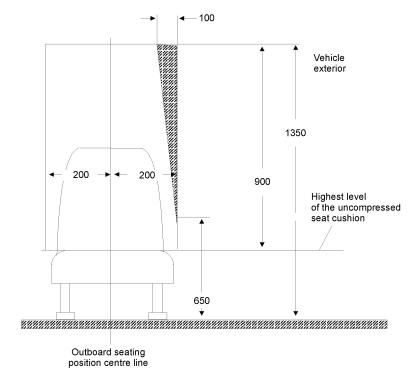
Figure 16 Permitted intrusion in lower part of passenger space
