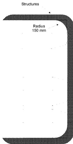
*Figure 18***Permitted intrusion of a wheel arch not extending beyond the vertical centre line of the side seat****(see Annex I paragraph 7.7.8.6.4.2.1)**
