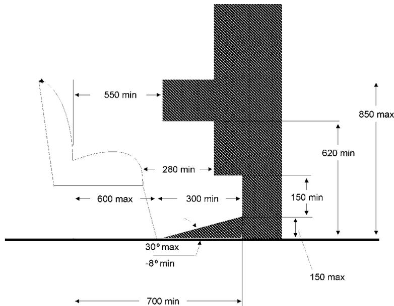
**▼B***Figure 14***Permitted intrusion into space above seat****Transversal section of the minimum free space above a seating place adjacent to the wall of the vehicle****(see Annex I paragraph 7.7.8.6.3.1)**
