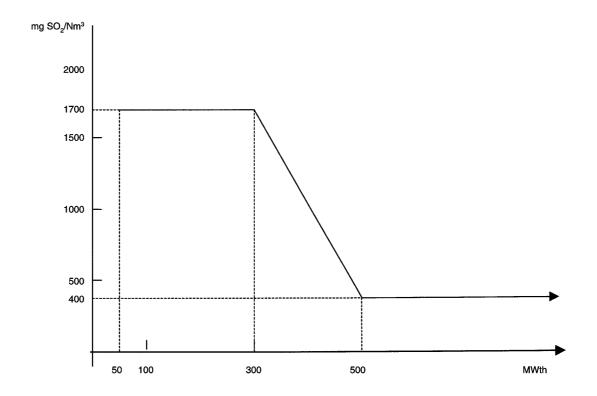
B.  $SO_2$  emission limit values expressed in mg/Nm³ ( $O_2$  content 3 %) to be applied by new plants pursuant to Article 4(2) with the exception of gas turbines
