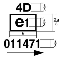
The device bearing the EC component type-approval mark shown above is a direction indicator lamp of category 4, type approved in Germany (e1) purusant to this Directive (01) under the base approval number 1471, which may also be used in an assembly of two lamps. The arrow points towards the front of the vehicle.
