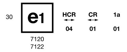
The above example corresponds to the marking of a lens intended to be used in different types of headlamps, namely:
