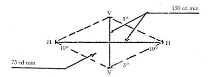
3.1. Intensities outside the axes shall be measured within the rhombus described by the extreme directions of measurement (see diagram above).
