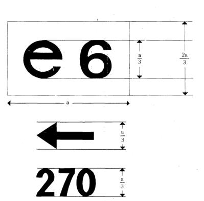
The device bearing the EEC component type-approval mark shown above is a device comprising a direction indicator lamp in category 2, a stop lamp, a rear position (side) lamp, a reflector in class I, and a rear fog lamp, EEC type-approved in Belgium (e 6) under the number 270. The arrow shows in what position this device, which can be mounted only on one side of the vehicle, is to be mounted. The arrow points towards the front of the vehicle.
