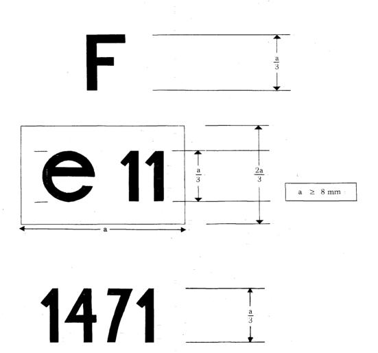
The device bearing the EEC component type-approval mark shown above is a rear fog lamp EEC type-approved in the United Kingdom (e 11) under the number 1471.
