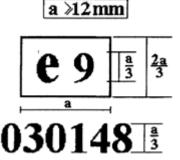
The exhaust system or component thereof bearing the above EC type-approval mark is a device which has been approved in Spain (e 9) pursuant to Directive 92/97/EEC (03) under the base approval number 0148.
