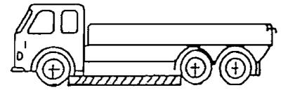
4.5.2. 'Ground clearance beneath one axle' means the distance beneath the highest point of the arc of a circle passing through the centre of the tyre footprint of the wheels on one axle (the inner wheels in the case of twin tyres) and touching the lowest fixed point of the vehicle between the wheels.
