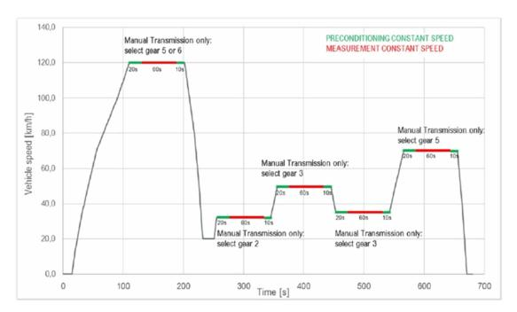
Each constant speed phase has a duration of 90 seconds, subdivided into 20 seconds for speed and emission stabilization, 60 seconds during which OBFCM measurement takes place and 10 seconds preparation time for the driver for the upcoming driving manoeuvre.
