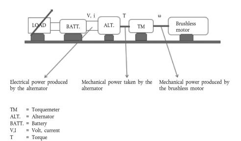
In figure 1 an overview of the test bench configuration is given. The alternator transfers the mechanical power of the brushless motor into electrical power. The brushless motor generates an amount of power which is defined by the torque (Nm) and by the rotational speed  $(rad.s^{-1})$ . The torque and the speed are to be measured by the torque meter.
