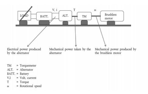
In figure 1 an overview of the test bench configuration is given. The alternator transfers the mechanical power of the brushless motor into electrical power. The brushless motor generates an amount of power which is defined by the torque (Nm) and by the rotational speed (rad.s<sup>-1</sup>). The torque and the speed are to be measured by the torque meter.
