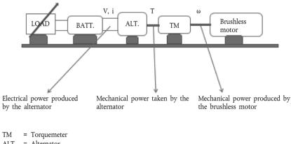
$\begin{array}{lll} ALT. &=& Alternator \\ BATT. &=& Battery \\ V,I &=& Volt, \ current \\ T &=& Torque \\ \omega &=& Rotational \ speed \\ \end{array}$
