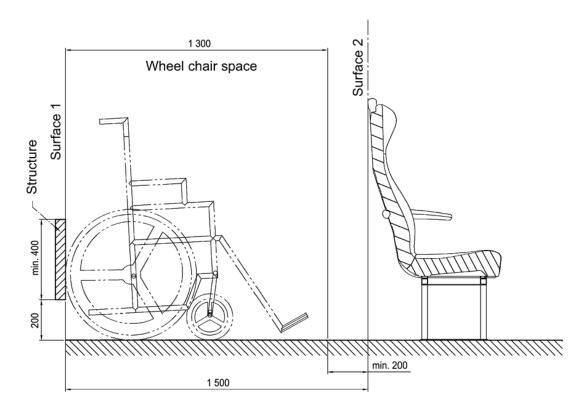
Tip-up or folding seats may be installed in the wheelchair space but, when in the stowed position, shall not encroach on the dimensional requirements of the wheelchair space.
