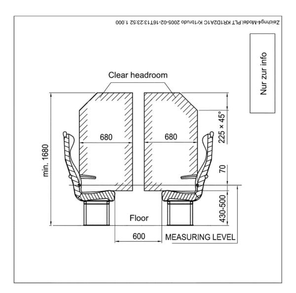
Where reclining seats are fitted, the dimensions shall be measured when the seats are in their fully upright position.
