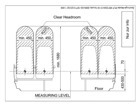
The top of each priority seat cushion shall be between 430 and 500 mm above floor level at the front edge of the seat. The clear headroom above each seat shall be at least 1 680 mm from floor level (see figure 2), except on double-decker trains on which luggage racks are provided above the seats. In such case a reduced headroom of 1 520 mm is permitted for priority seats underneath the luggage racks, provided that at least 50 % of priority seats maintain a headroom of 1 680 mm.
