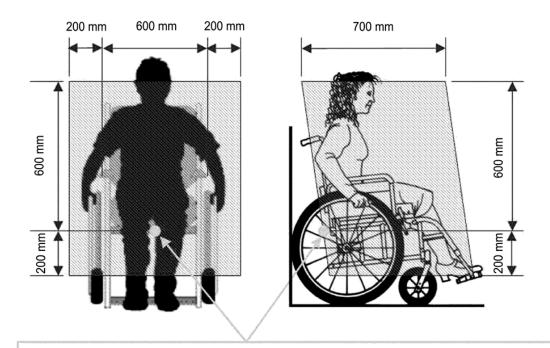
Seat Reference Point (480 mm +/- 20 mm above floor and 350 mm +/- 20 mm forward of the structure)
