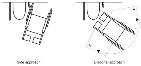
In front of the toilet seat there shall be a minimum clear space of 700 mm as shown in figure 8b.
