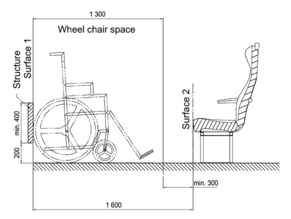
If surface 2 is the front edge of a passenger seat cushion in a facing arrangement and if this seat can be occupied by a passenger, the minimum distance shall be not less than 300 mm.
