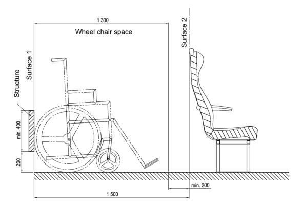
Tip-up or folding seats may be installed in the wheelchair space but, when in the stowed position, shall not encroach on the dimensional requirements of the wheelchair space.
