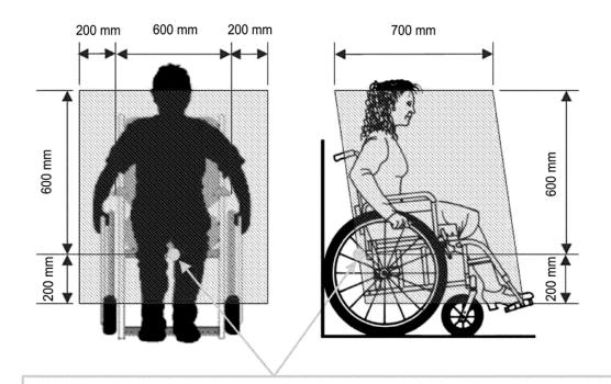
(480 mm +/- 20 mm above floor and 350 mm +/- 20 mm forward of the structure)
