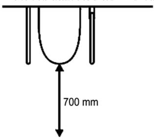
A horizontal handrail that complies with the dimensional requirements in the clause above shall be provided at each side of the toilet seat. The handrail on the wheelchair accessible side shall be hinged in such a way so as to enable an unobstructed transfer for the wheelchair user to and from the toilet seat, see figures 9 and 10.
