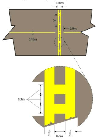
signifies a holding position other than that closest to the runway beyond which no part of a flying machine or vehicle must project in the direction of the runway without permission from the air traffic control unit at the aerodrome during the notified hours of watch of that unit.
