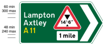
2027 Direction to a primary route along which there is a low bridge
