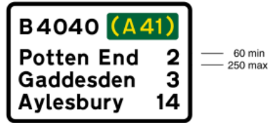
2128 The number of a non-primary route leading to a primary route with destinations and distances
