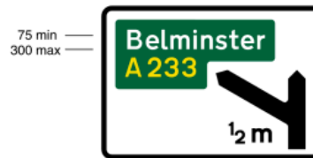
2101.1 Grade separated junction ahead of a non-primary route and a primary route
