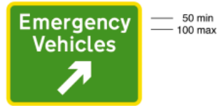
2709 Direction of route or junction ahead leading to a route for emergency vehicles to an emergency services incident point
