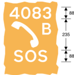
2715 Back of emergency telephone box
