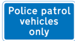
829.6 Waiting place at a lay-by or observation platform for police vehicles only
