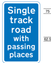
821 Road ahead only wide enough for one line of vehicles, but has passing places at intervals
